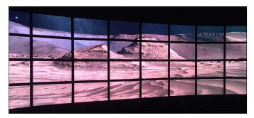
Fig. 6: Browsing the surface of Mars in a clustered environment rendering on the power wall at the University of Utah. The system uses eight rendering nodes, each connected to four screens.
