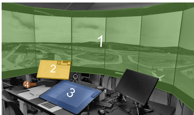
Fig. 6 The RTC simulator used for the evaluations, including annotations for the different components. 1: Animated 3D Tower View of the runway. 2: Radar display for the airspace surrounding the airport. 3: Touch screen for interacting with the electronic flight strips. 4: Headphones used to listen to the sonification
