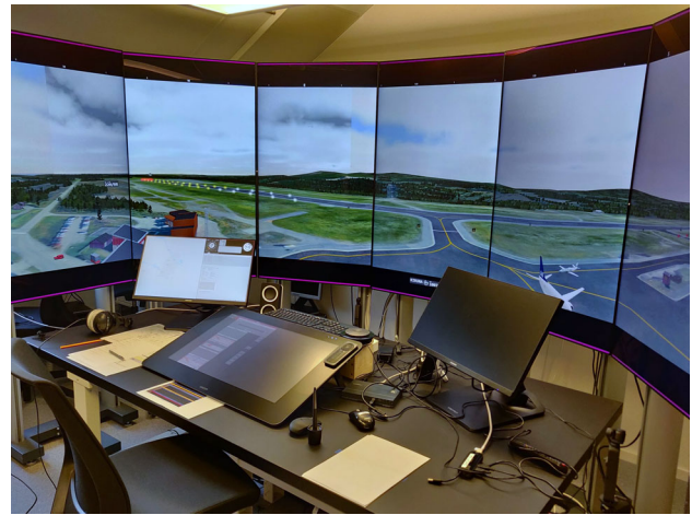
Fig. 1 The remote tower center (RTC) simulator where the sonification was integrated and evaluated
